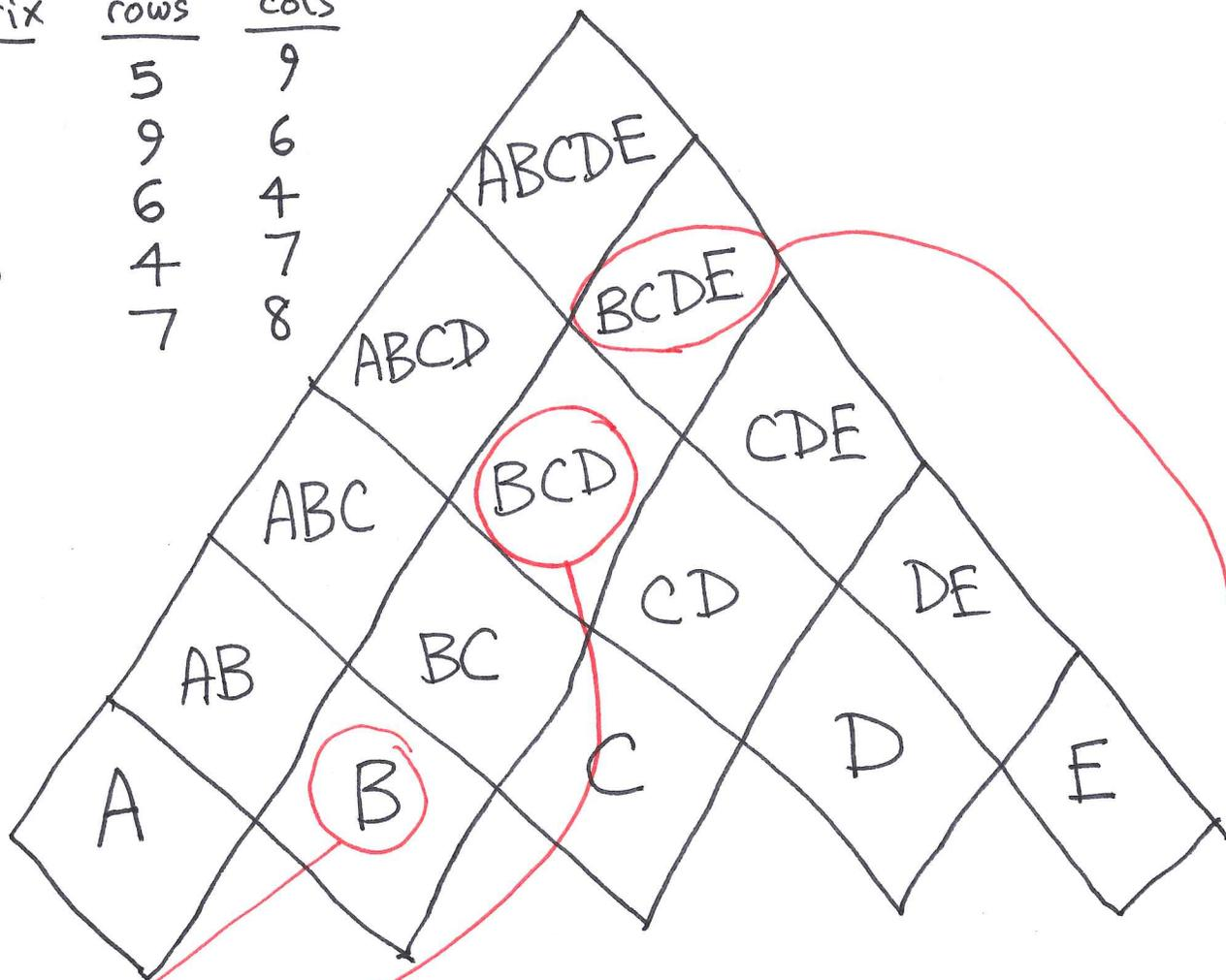
This square BCD contains the minimum number of operations required to produce the matrix  $B \times C \times D$
