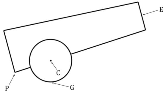
G is the point on the ground where the wheel rests. Its coordinates are (xg, yg). C is the exact position of the axle, its coordinates are (xc, yc). P is the easiest point to start drawing the body of the cannon from, coordinates (xp, yp). E is the point where the ball pops out when it is fired, coordinates (xe, ye).
