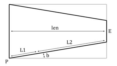
This is a simplified picture of the body of the cannon shown with its "bounding box". The point is to illustrate the difference between the real length of the cannon (len) and the sum L1+L2.
