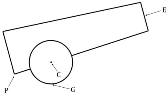
G is the point on the ground where the wheel rests. Its coordinates are (xg, yg).
