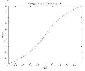
Figure 11: Soft clipping transfer function for K = 1, note the smoothness.
