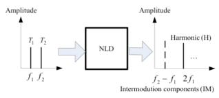
Figure 4: Intermodulation distortion caused by a nonlinear device (NLD).
