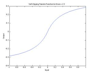
Figure 12: Soft clipping for K = 2.5, note how the curve flattens much faster than the previous transfer function.
