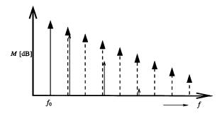
Figure 7: Spectrum of the output of both a full-wave rectifier and full-wave integrator. The solid arrow at  $f_0$  represents the input spectrum, arrows at  $2 f_0$ ,  $4f_0$ , etc., represent the output spectrum for the full-wave rectifier and dashed arrows at  $2f_0$ ,  $3f_0$ , etc., represent the output spectrum for the full-wave integrator.
