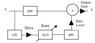
Figure 9: Tunable virtual bass plug-in design.
