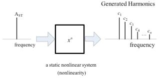
Figure 3: NLD measurement by introducing a single sinusoid into the system.
