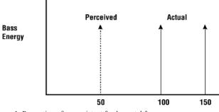
Figure 1: Perception of non-existent fundamental frequency.
