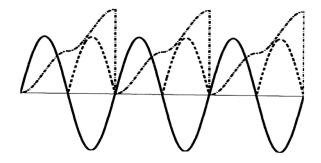
Figure 6: Output of a full-wave integrator at different stages. The dashed line is obtained by full-wave rectification, the dashed-dotted line by full-wave integration.
