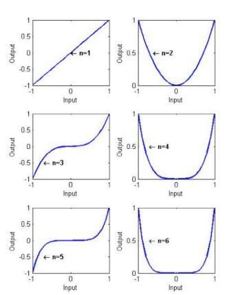
Figure 8: Linear and nonlinear system transfer function plots from n = 1 to n = 6, where n is the order of nonlinearity.
